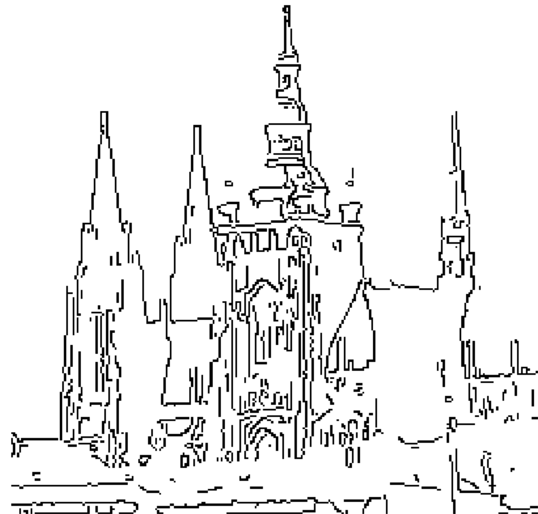
hysteresis high threshold 70, lower 10
